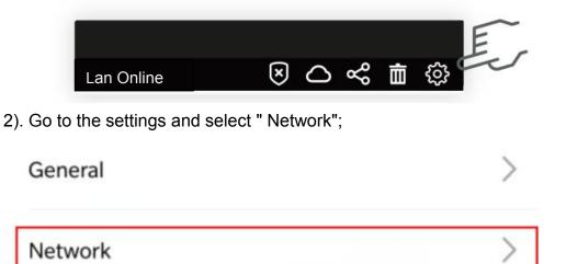
3). After entering the interface, click "Change to WiFi station mode" at the bottom of the interface;
