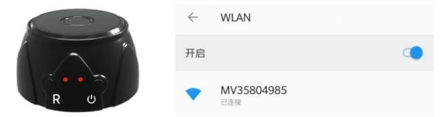
4). When the mobile phone is connected to the camera hotspot, open the APP(V380 Pro) pull-down interface to refresh the data and automatically add the device.
