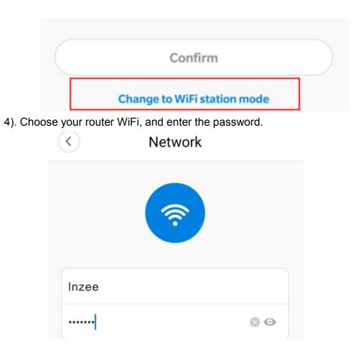
5).After the setting is completed, the device light switches from red to blue, then the device is in remote mode. The process of the remote mode setting needs to wait for two minutes.
