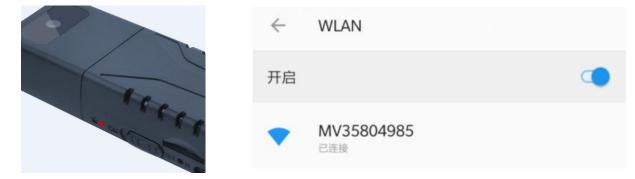
4). When the mobile phone is connected to the camera hotspot, open the APP(V380 Pro) pull-down interface to refresh the data and automatically add the device.
