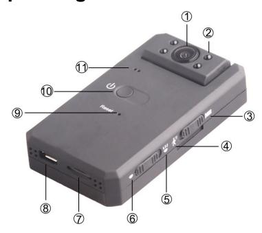
①Lens ②IR LED ③Video ④Motion detection Mode ⑤IR LED-ON ⑥IR LED-OFF ⑦TF CARD ⑧USB ⑨Reset ⑩Power key ⑪LED
