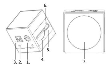
1.Power button; 2.M-Mode button; 3.LED; 4.TF Card; 5.USB; 6.Reset button; 7.Magnet
