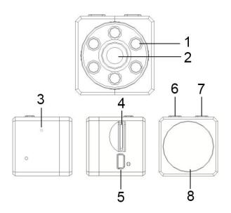
1.IR-Infrared night vision light; 2.Lens; 3.LED indicator; 4.TF/SD card slot; 5.USB port;6.M-Mode button; 7.Power button; 8. MagnetNote:
